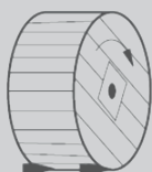
The drum should be stood upright, using wedges in the heels of the flanges.
